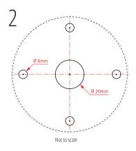
If you require cable management for charging, please punch centre of 20mm diameter hole. Drill pilot hole first to ensure it remains central to outer 4 fixing holes. Finally, bore a hole of approximately 20mm in diameter to allow USB end of charge/sync cable to pass through.
