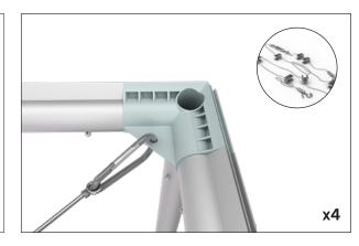
**Step 4:** Move to the center of cable and hand tighten turnbuckle to remove any remaining slack. Do not over tighten.
