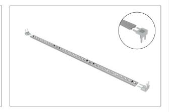
**Step 4:** Join vertical side frames to top and bottom horizontal frames.
