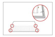
**Step 7:** Connect the feet by inserting into the bottom holes of frame and pressing firmly.
