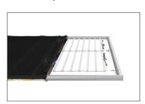
**Step 2:** Take out the LED Light Array and gently unroll on the ground with lights face down. **Warning!**Do not drag lights across ground or it could break the LED lights.
