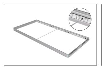
**Step 8:** To install a graphic start by inserting one eSEG™ Fabric Print into 4 corners of frame by pressing silicone into frame edge.
