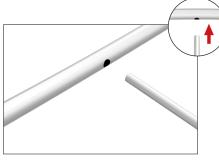
**Step 6:** Add shelves to frame. Position and level shelves on frame before tightening clamps down with hex tool.
