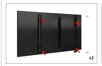
**Step 4:** Insert base plate pole through front of graphic.
