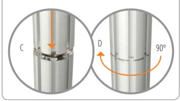
Repeat for remaining base and posts to complete assembly of uprights.
