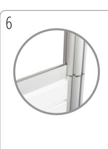
Slot clamps of middle 750mm profile into post channels and slide profile onto top of slatwall panel. Close T-Loc levers to secure.
