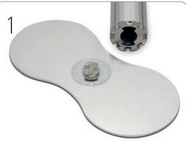
Place base plates on the floor, position lower posts centrally over male fitting of base plate (A), and rotate until assembly drops into position, continue rotating clockwise through 90° to secure (B).
