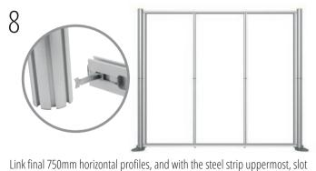
Link final 750mm horizontal profiles, and with the steel strip uppermost, slot onto top of vertical rails and channel of posts. Close remaining T-Loc levers to finish assembly of the framework.
