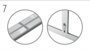
Clamp the middle vertical rails with twin steel fixing strips, halfway across the joins of 750mm bottom horizontal profiles.
