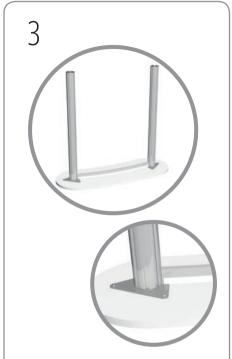
With the steel fixing strip of curved profile adjacent to counter top, slide first curved profile between posts, in channels aligned to cut out of triangular fixing plates.
