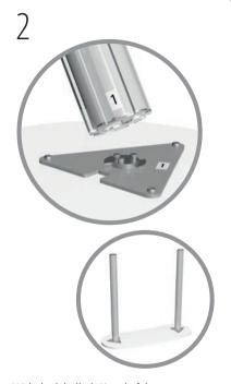
With the labelled '1' end of the post towards the counter top, position female fitting of post centrally over male fitting of triangular fixing plate. Rotate until post drops into position, continue rotating post clockwise through 90° to secure. Repeat for second post.
