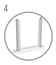
Assemble vertical profiles to the curved profile ensuring that the graphic fixing strip is adjacent to the post and facing forward (convex side).
