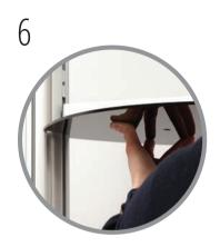
Ensuring the black acrylic is lowermost, slide and raise second assembly into the same post channels as the previous enclosure until the T-Loc clamps come into contact with the bottom of the pre-installed locator bars of the upper posts. Close T-Loc levers to secure in position.
