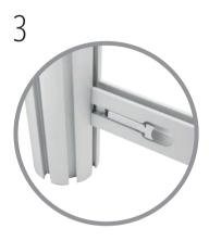
Position post assemblies facing one another with aligned shelf brackets inwards. Connect post assemblies by attaching one of the straight 616mm profiles to the bottom, parallel to the shelf brackets. Slot clamps of profile into post channels and close T-Loc lever to secure.
