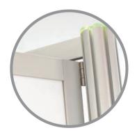
Slide third/final hinge with connector bars into same channel of post and door vertical profile. Position hinge near top of door and tighten four screws to secure. Finish door assembly by positioning straight 750mm profile flush with the top of the posts, and tighten grub screws to secure.
