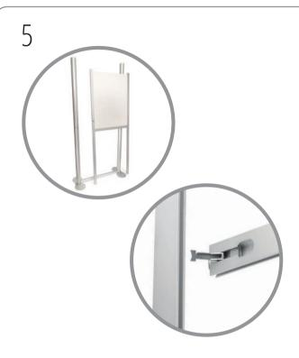
Slide upper and lower rigid panels into channels of profiles. Secure panels in position by assembling top and bottom horizontal 654mm straight profiles.
