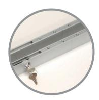
Assemble two of the 950mm straight profiles by inserting half of connector bar into one end of profile, tighten 2 grub screws, and assemble upper 950mm straight profile. Repeat process for other two 950mm straight profiles.
