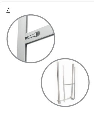
Affix middle horizontal 654mm profile (with handle on front), halfway between verticals of door. The profile is affixed by closing T-Loc levers so secured into channel of profiles. Ensure lock lever is located on the outside of the door assembly.
