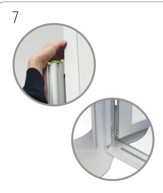
Raise door assembly and slide connector bar of second hinge into same channel of post as first hinge. Position bottom of door frame over first hinge and rest assembly on door threshold. Tighten two screws in frame to secure.
