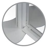
Carefully place door threshold onto base plates between posts. Insert wide section of first 'L' shaped connector into end of door threshold and tighten grub screws to secure. Repeat process for opposite post.
