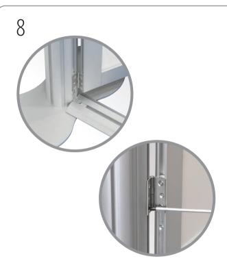
Raise door so there is an approximate 25mm (1 inch) gap between underside of door frame and top of door threshold. Tighten screws of hinges in post channel to secure.
