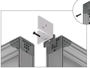
**Step 4:** Complete install of connectors by pushing the DNA Panel into place and instaling screws top and bottom.
